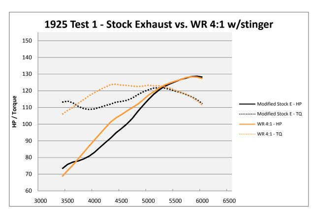
The WR 4:1 header with the 10" stinger/resonator provided an amazing boost in the mid range torque – right in the driving range. Some low end torque is sacrificed (below 3800rpm due to the lack of back pressure), and above 5800 (due to the resonating length of the primaries).
