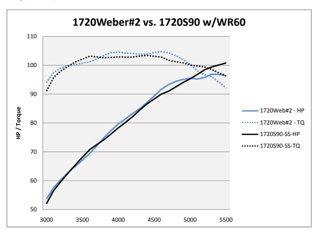
This comparison shows two things, the boosted mid range available with the Weber air horns, and the boosted top end performance available with the WR60 camshaft.
