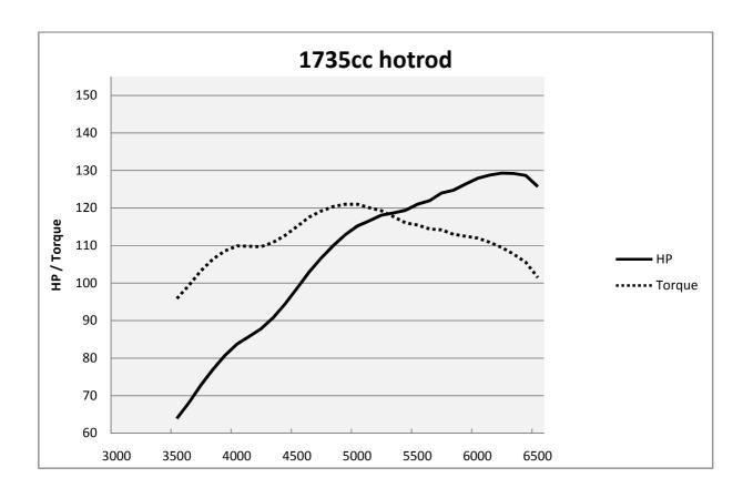
This was the first engine we dyno tested at Carobu. The intakes were ported to flow into the valves, and the chambers were unshrouded, but the intake manifolds at the gaskets were kept stock. Peak flow at .500" was later tested at 176cfm. The long primary pipes of the WR 4:1 header gave an excellent boost to the mid range torque, but with a VERY sporty sound.
