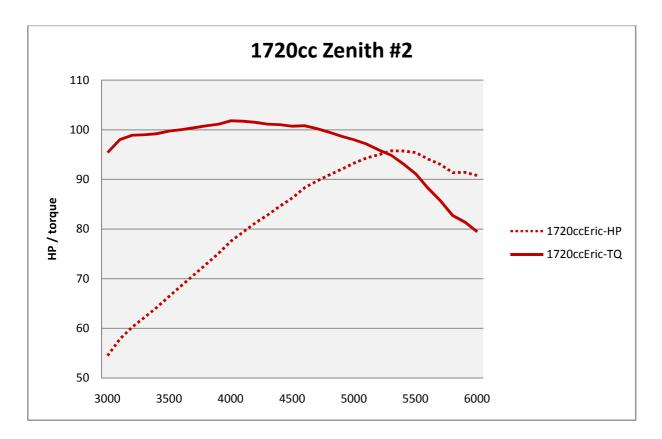
This engine was as responsive as the #1 version but pulled the power much further. The bigger cam definitely helped with the top end. It's obvious that more intake lift and duration is what engine #1 needed. The added lift of the late rockers helped a lot. The mild cam does help the very low end, and if around town driving and maximum fuel economy is what you're after this might be the cam you want.
