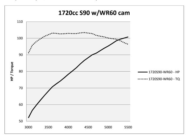
The next graph compares a basically stock 1720cc SC Solex#2 and the 1720cc S90 with WR60 camshaft. The smaller exhaust valves don't seem to help the SC.
