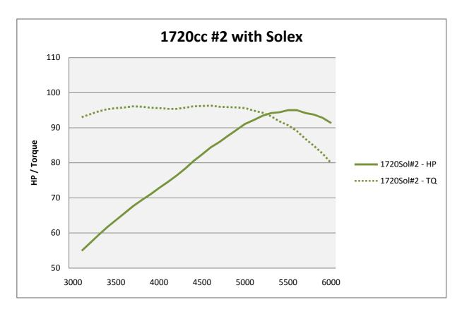
Comparing this test to the #1 test engine shows the advantage of the "Super/S90/SC/912" camshaft. It's much better suited to the larger Solex carbs than the milder low lift cam.
