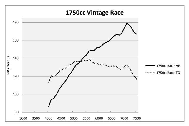
This was an incredibly strong runner. The big cam combined with the big carbs moved the torque and hp curve way up. We couldn't load the dyno below 4000 or the engine would stall. It would be interesting to explore other possibilities with a "legal" vintage race engine. This one ended up going to a customer in the UK who was going to use it for "track days" so the 1750cc size and the 48mm carbs weren't a problem. The bump in the curve at 6900RPM was the result of the reverse cone megaphone.
