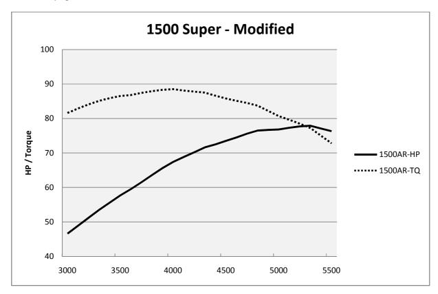
Porsche listed the power output of the stock 1500S at 70HP@5000 /80ftlbs@3600. Our torque and HP peaks definitely moved up, but not at the expense of low end performance (the 80ftlbs were already there at 3000)
