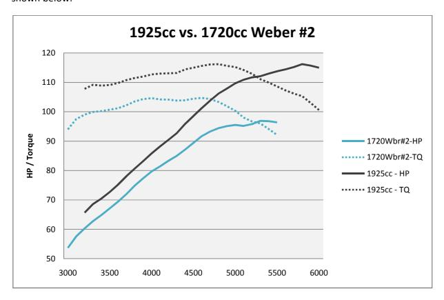
You can see from the graph that the 1925cc engine is already beating the 1720s maximum torque at the beginning dyno test rpm of 3200. This graph shows that engine size is the best way to increase power.
