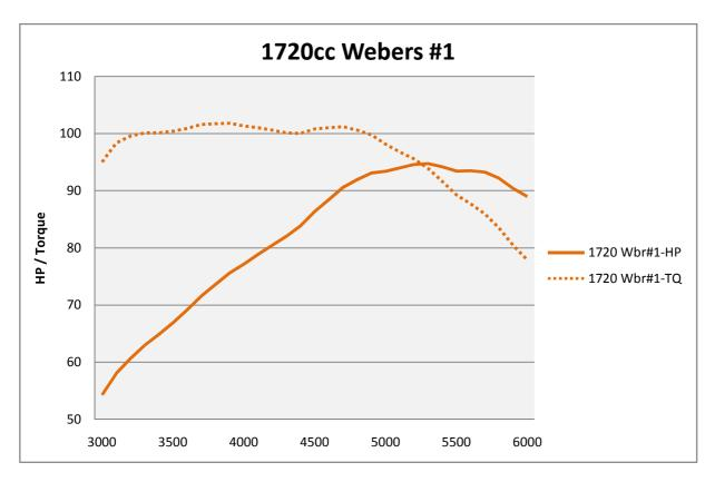
This engine was a strong runner which provided excellent low end and midrange with a basically stock power curve. The torque curve was almost flat from 3700 to 4700.
