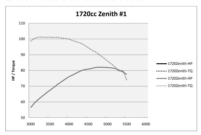
This engine was an excellent runner with much improved low end torque. Since it started life as a 1600 Normal, the owner was happy with the added torque, but the power fell off very quickly due to the short duration cam, lower lift early rockers, and Zenith carbs.
