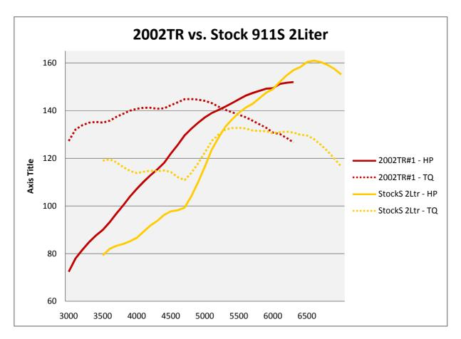
The 2Ltr 911S has the advantage of a bigger cam, higher RPM, and the added cylinder filling of 6 cylinders, but can't match the power of the 4 cylinder 2002TR until 6K. It will be interesting to compare a 2002TR with a hotter camshaft and free flow exhaust.
