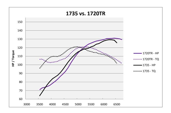
As you can see in the graph, the tuning affect of the long primaries and the taller air horns boosts the torque between 3500 and 5500rpm, but the TR set up with the WR Sport Exhaust and the stock Weber 2.25" air horns and air cleaners are much more reasonable for street use, and also boost power above 5000rpm. We also tried the TR engine without the K&N air cleaners and recorded no gain in power.
