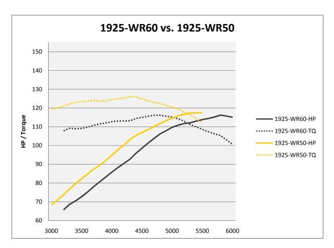
You can see from the chart that the new camshaft provided a real boost to the bottom end and mid range. We limited testing rpm to 5500 but the engine would easily load with full throttle at 2500 which is usually a problem for a most 356 engines. The engine hasn't been tested in the car as of yet, so that part of the evaluation will have to wait.
